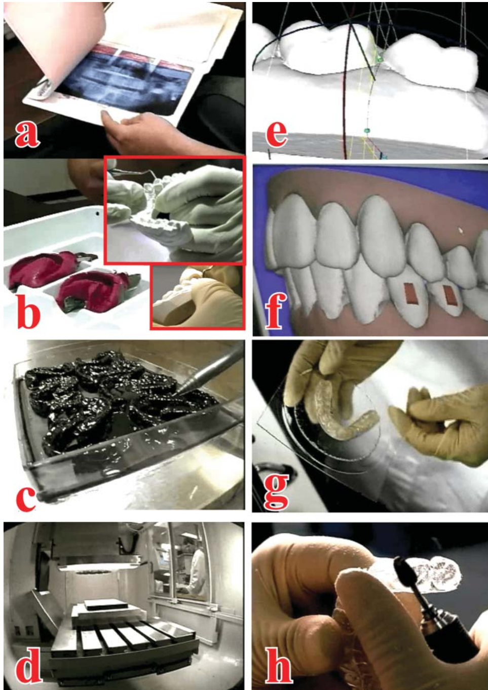
Figure 6 (a) Initial treatment planning with patients' photographs and radiographs are sent to Invisalign® laboratories. (b) Impressions are converted into positives (plaster models) and checked for quality. (c) In the laboratory, models are first coated with protective shells, and encased in a mixture of resin and a hardener. (d) After chemical setting, they become blocks of hardened resin with many plaster models inside. Each tray is placed in a destructive scanning machine. (e) Each 3D model is constructed from about 300 2D scans. Graphic designers cut out each tooth and save it as a separate geometric unit. (f) Once the teeth are separated and re-assembled back into the arches, the designers create a final set-up of what the patient's teeth will look like when the treatment is completed. (g) For each stereolithographic constructed model (which represents a treatment stage), a clear Invisalign® aligner is created by heat. (h) These aligners are trimmed, polished, cleaned and finally sent to the prescribing orthodontist.
